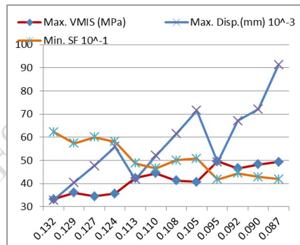
Figure 8: Graph Represents of Result for North America weight on the car seat of 791.667N
