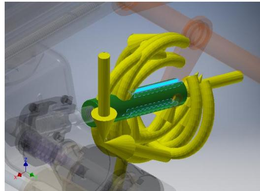
Figure 2: Diagram of loading conditions on car seat height screw adjuster showing the reaction Force and Moment on Constraints
