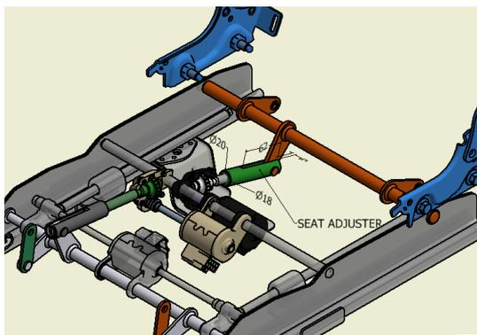
Figure 1: Diagram of car seat height screw adjuster
