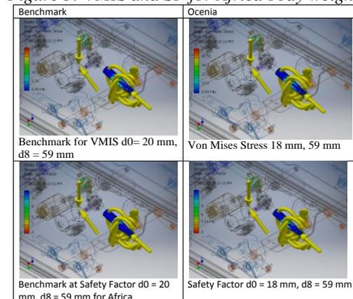
Figure 4: VMIS and SF for Oceania body weight
