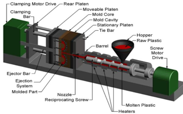
**Figure 2:** Isometric view and the sectional view of the mold of a Plastic Injection Molding Machine [13].
