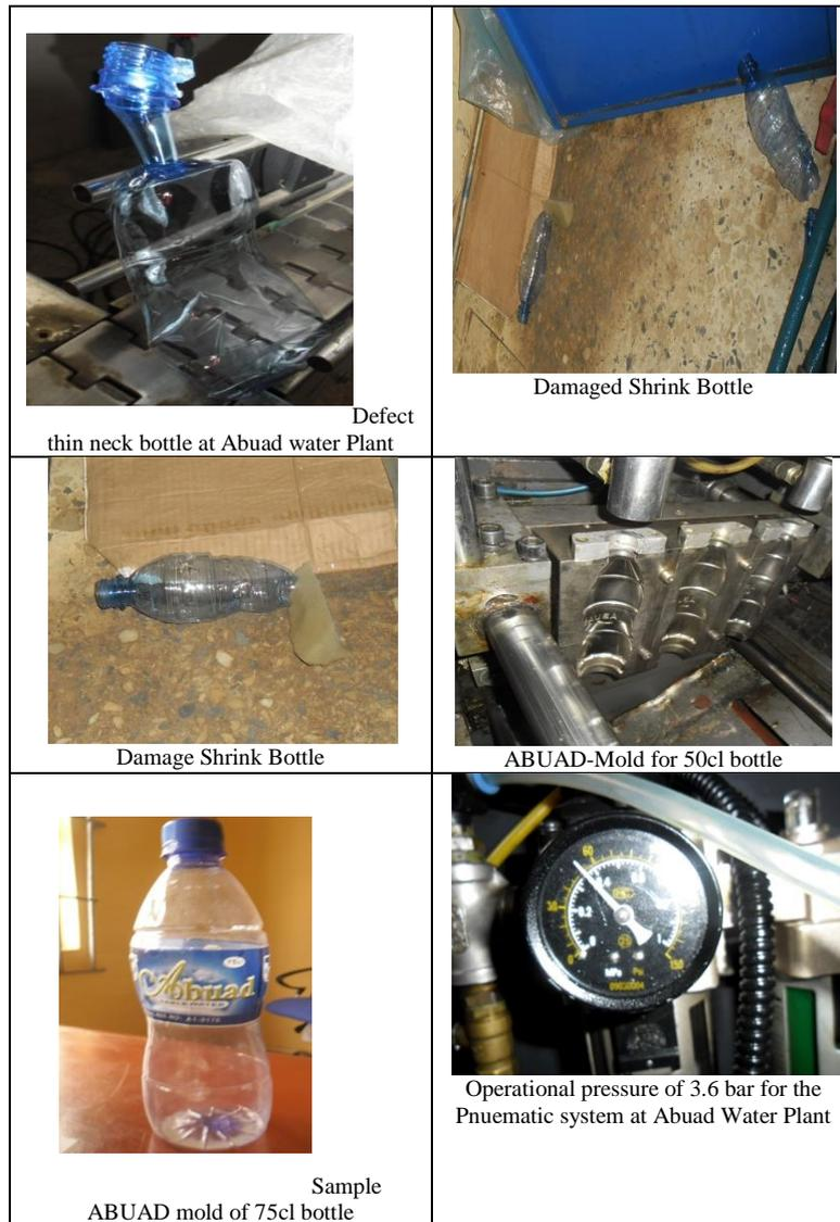
**Figure 1:** Investigation process into ABUAD Water Plant
