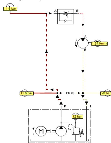
**Figure 4:** FluidSIM® setup and description after simulation using the Flow meter
