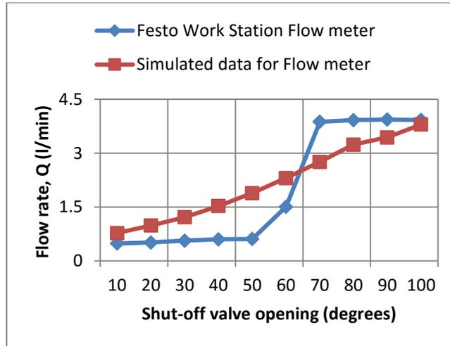
**Figure 7:** Simulated and Experimental Data graph for flow rate
