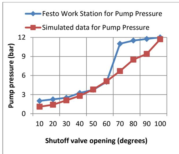
**Figure 8:** Simulated and Experimental Data graph for Pump Pressure
