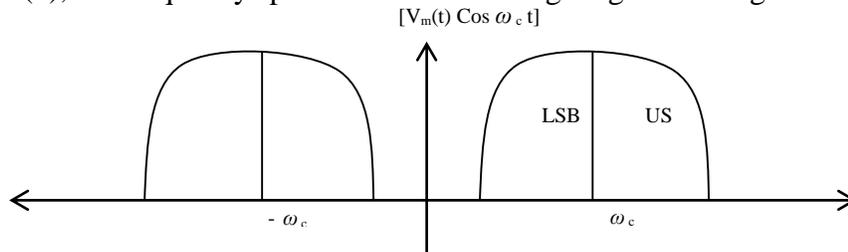
Figure 3: Frequency Spectrum Modulated signal
