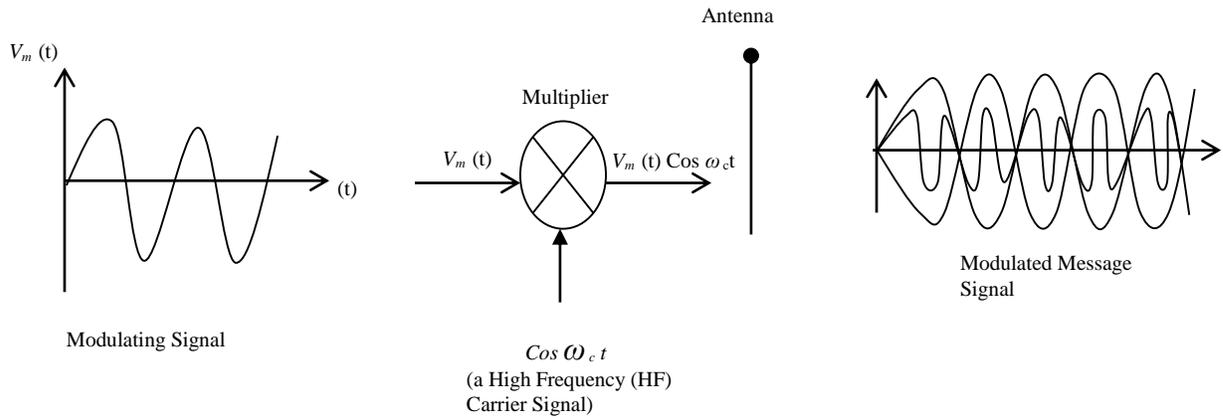
Figure 2: Amplitude Modulation
