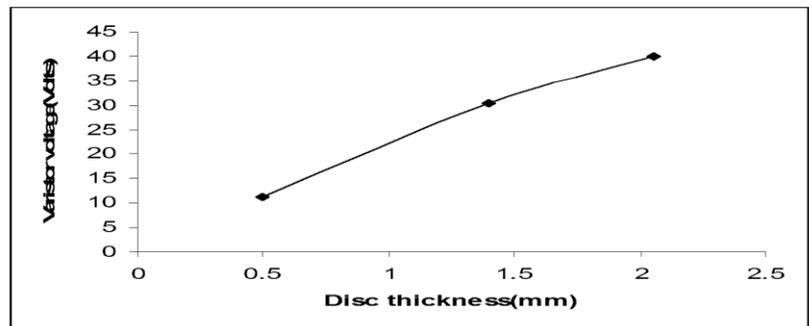
Figure 2: Dependence Of ZnO Varistor Voltage On Disc Thickness (Sample B).
