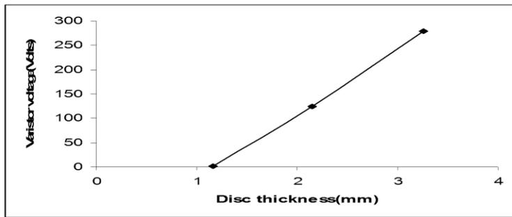
Figure 1: Dependence Of ZnO Varistor Voltages On Disc Thickness (Sample A).
