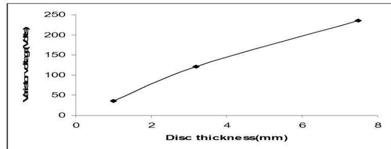
Figure 4: Dependence Of ZnO Varistor Voltage On Disc Thickness (Sample D).
