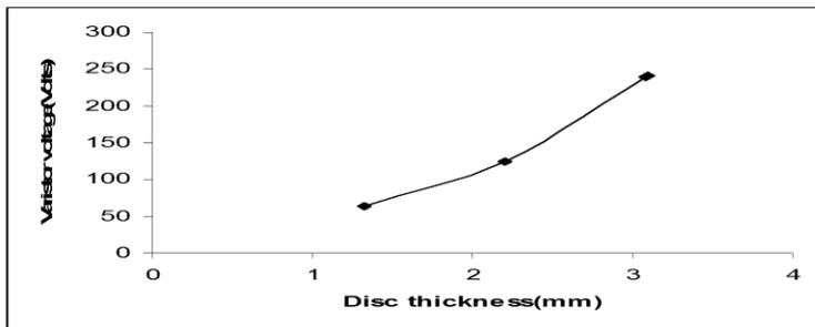
Figure 3: Dependence Of ZnO Varistor Voltage On Disc Thickness (Sample C).
