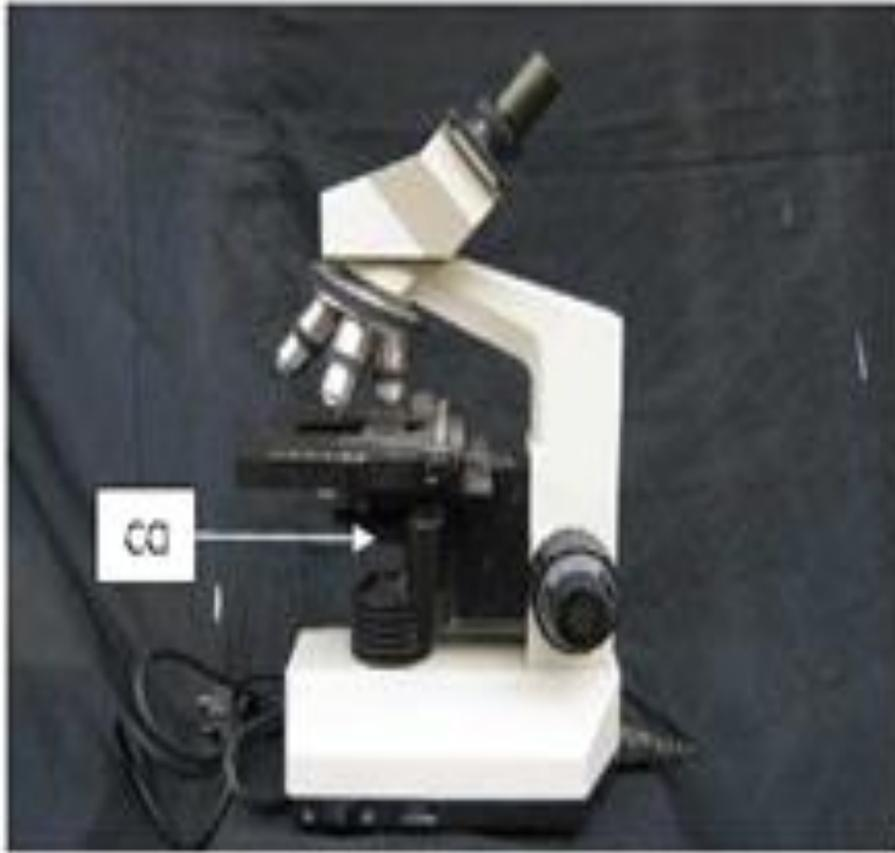
*Complex compound (CC) microscope with Condenser Chamber. (Photo from Bup Oyesiku Bryolab, 2011)*
