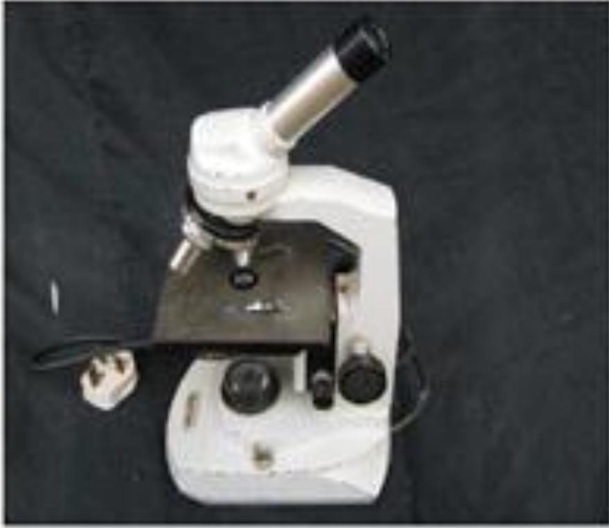
*Simple compound microscope without condenser lens beneath the stage. (Photo from Bup Oyesiku Bryolab, 2011)*
