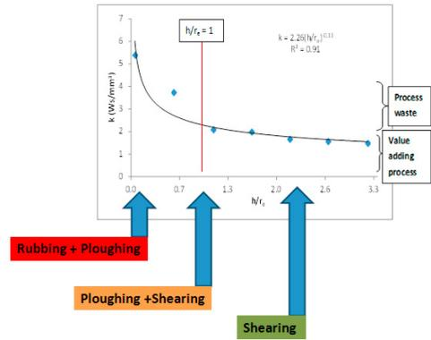
Fig. 3. Process mechanisms and specific cutting energy relationship
