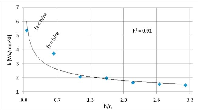
Fig. 2. Relationship between specific energy and  $h/r_e$  for AISI 1045 steel alloy.
