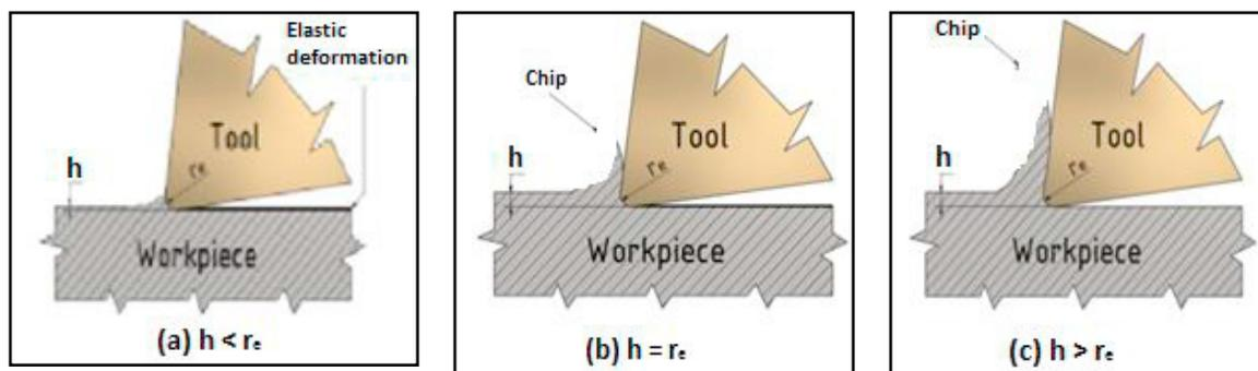
Fig. 1. Effect of un-deformed chip thickness ratio to the cutting edge radius in orthogonal cutting adapted from [9, 10] [22].
